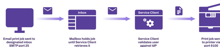
Figure 6: Email printing job flow using a Vasion Print VA-hosted Service Client and user validation against Active Directory or a cloud-based IdP.
