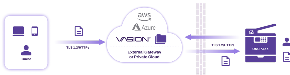
FIGURE 7: Web Print flow for guest users, detailing the process from document upload via a BYOD device to encrypted storage in Vasion's AWS, followed by release confirmation and the ONCP App downloading and printing the document.
